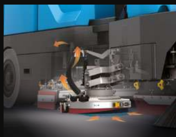
Side scrubbing brush with vacuum system
