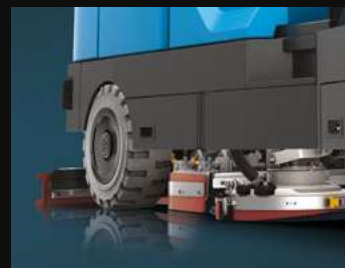
Super elastic front and rear wheels
