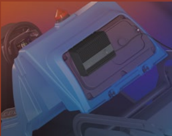
On-board battery charger
